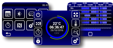
AirGENIO SUPERIOR - Main control functions
